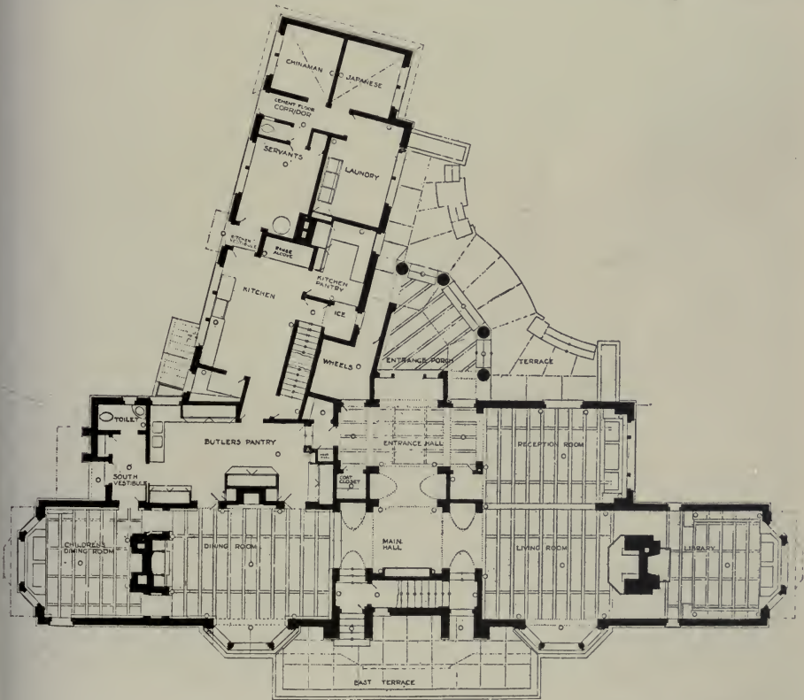
FIG. 1. FIRST FLOOR PLAN.—THE HOUSE OF MR. LIVINGSTON JENKS.
